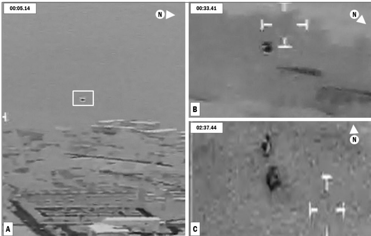
Figure 3: These stills demonstrate how the changing view angle from the sensor to the objects influenced their perceived behavior as the aircraft gained altitude. They appear to be one object from a low angle and a low magnification, as shown in Image A at 00:05.14. The objects appear distinct from one another from a steeper viewing angle and moderate magnification, as shown in Image B at 00:33.41. Image C, at 02:37.44, shows the objects from a high angle and increased magnification, clearly showing object separation from a more top-down perspective.
